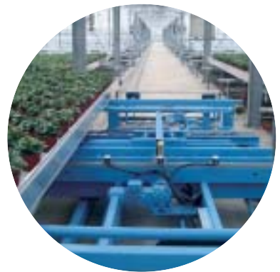
Automatic single or multi-layer transport robots for the loading and with drawal of benches
