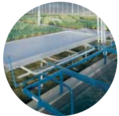
Track-guided, manual transport trolley with interlocking system
