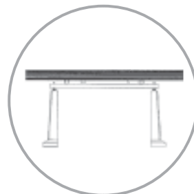
Concrete posts with recesses for traverse for heating pipes to be mounted in the ground (into concrete)
