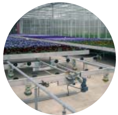
Stationary transport track with or without pneumatic lifting elements
