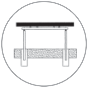
Model "B": galvanised steel posts with or without a traverse for heating pipes, for mounting into concrete (in the ground)
